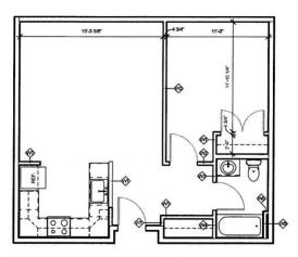
NOTE: DIMENSIONS IN THIS PLAN ARE TO THE FINISH FACE OF THE WALL
